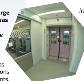
In the vestibules providing access to the carriages, the accumulation of ice and snow is a source of risk for passengers, the ground becoming slippery. Heating cords installed in the floor eliminate this danger and also makes it possible to increase the comfort of passengers who stay in the vestibules during the trip.
