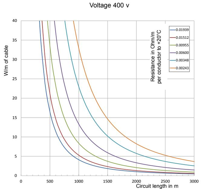
**Circuit lengths for 3 conductors star coupling**
