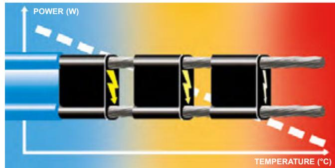
**NB :** unlike the other heating elements, it is impossible to check that a self-regulating cable is operating correctly by measuring resistance with an ohmmeter. This can be done instead by measuring the voltage/current.
