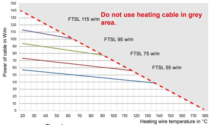
The curve above presents the power in w/m in comparison to the heating wire temperature. The heating cable must be covered 100% with an adhesive aluminium and installed on a metallic support. Consult our technical department for any informations.
